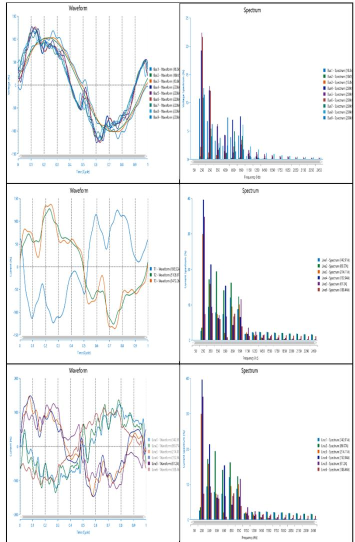
Fig. 6 Harmonic analysis plots for buses, transformers and transmission lines for typical IEEE 6 pulse 1 model.
