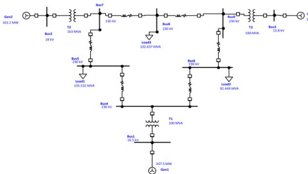
Fig. 1 Nine-bus system diagram.
