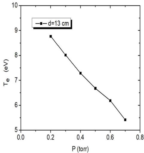
Fig.(4) Changing electron temperature with a change in pressure at constant power and a separation distance between the electrodes 13 cm
