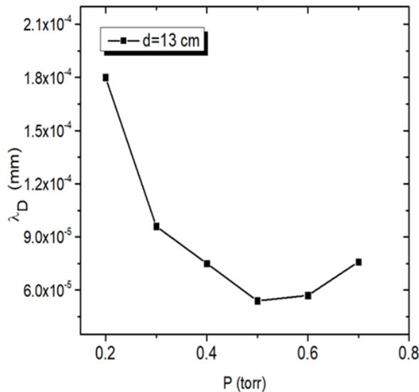
Fig.(7) Changing Debye length with a change in pressure at constant power and a separation distance between the electrodes 13 cm
