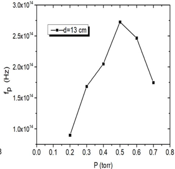
Fig.(8) Changing the plasma frequency with a change in pressure at constant power and a separation distance between the electrodes 13 cm.
