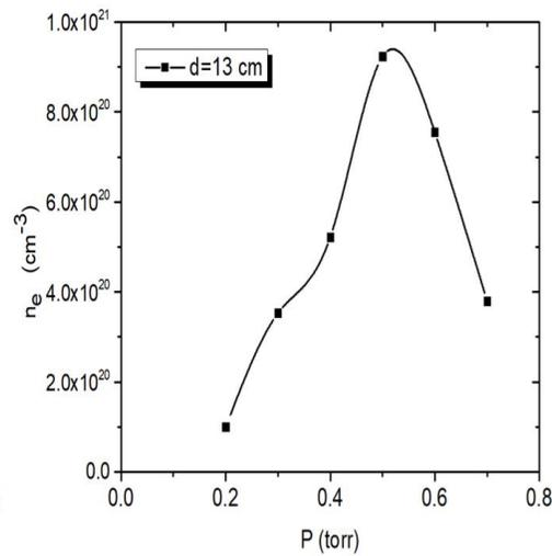
Fig.(5) Changing the electron density with a change in pressure at constant power and a separation distance between the electrodes 13 cm.
