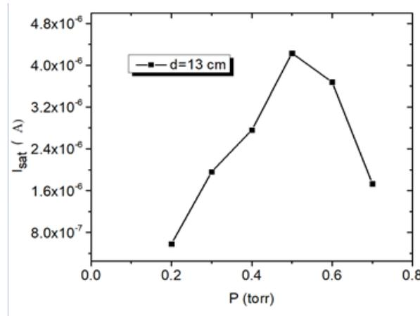
Fig. (6) the change of ionic saturation current with pressure.
