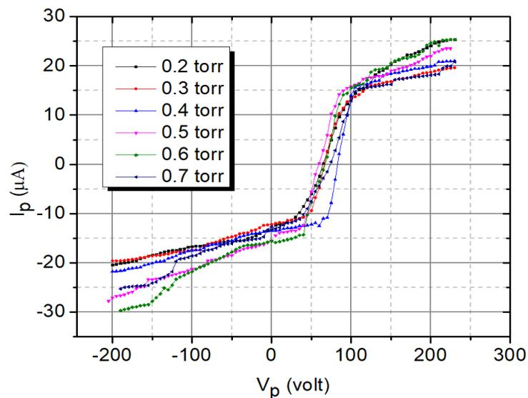
Fig. (3) Double probe I-V characteristics at different air pressure and the inter-electrode distance is 13 cm at constant power 0.6 watt.
