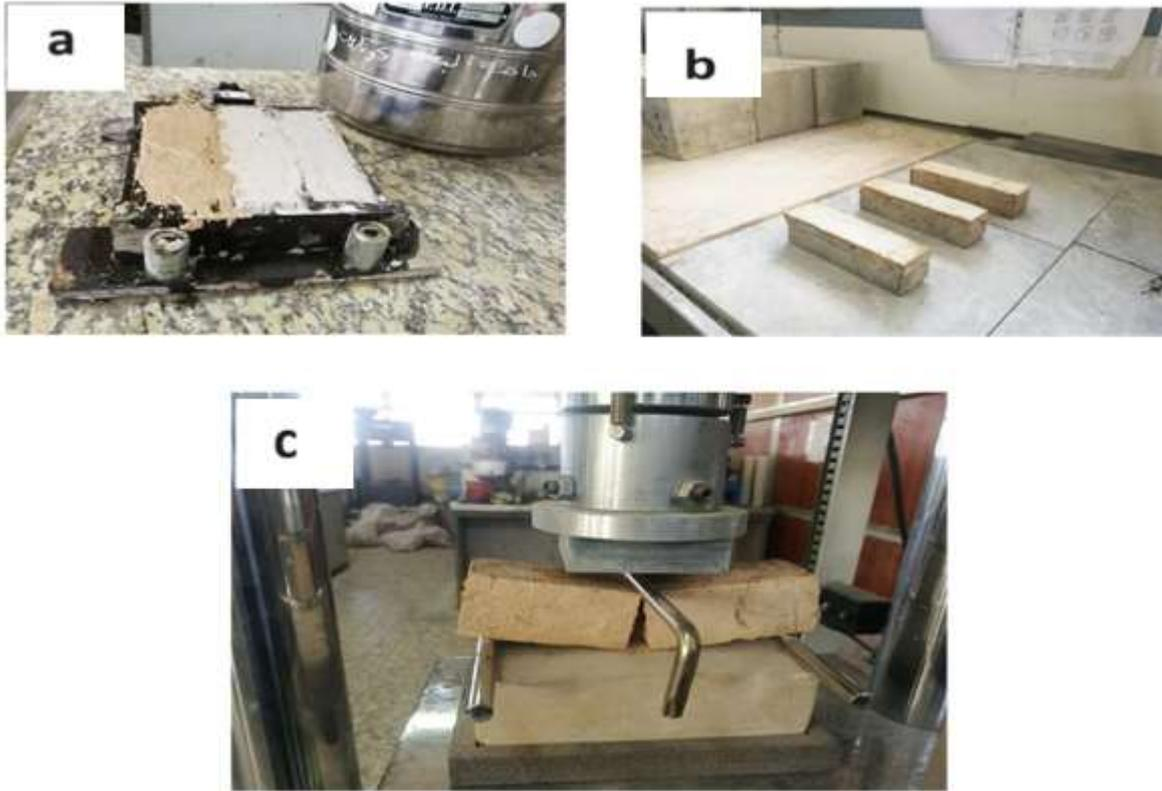
Plate 2: a- Dimension cube for tests, b- Rigid dimension cube for tests, and C- panel composite flexural test
