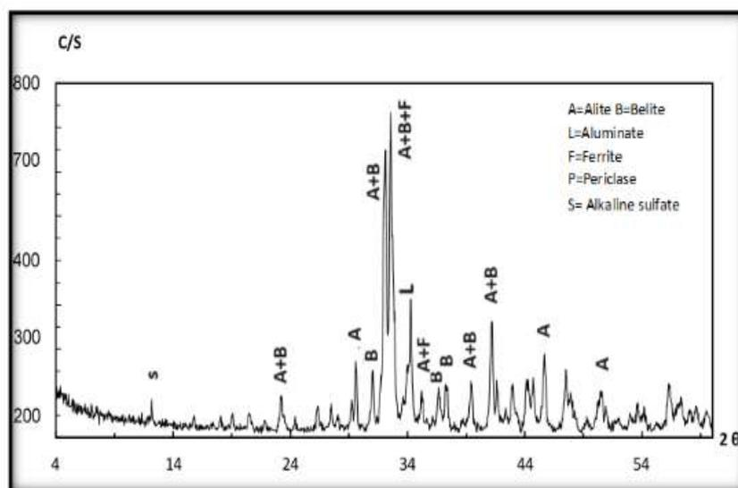
Fig. 5 The XRD patterns for produced clinker
