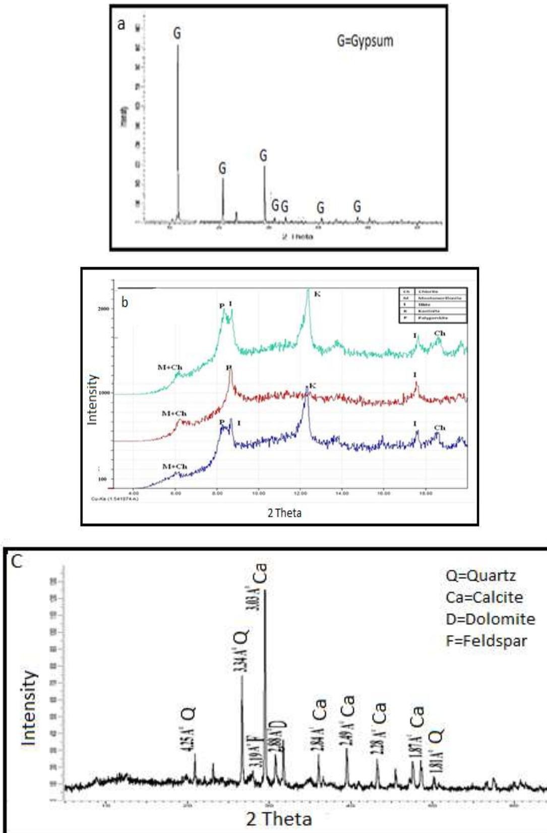
Fig. 4. X-Ray diffraction patterns a- Gypsum of Fat'ha Formation b- Clay minerals of Injana Formation c- Non clay minerals of Fat'ha Formation
