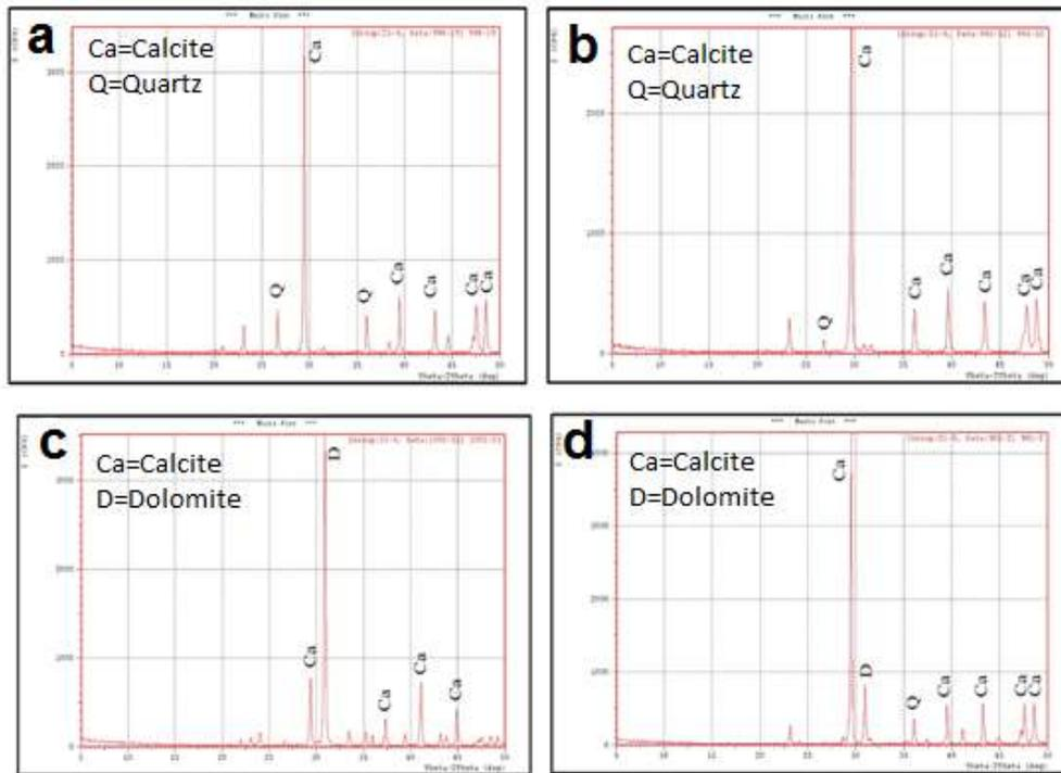
**Fig. 3. X-Ray diffraction patterns of limestone**
