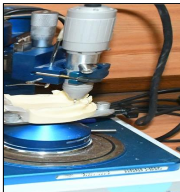
Figure (2): Milling Machine Drilling the Master Model by Pilot Drill.
